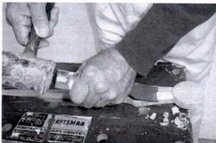
Figure 49a. Using a chisel to form the motif on a Chase paddle. Below-using a small spokeshave to continue forming the motif.
